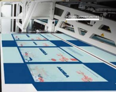
on a sheet before die-cutting and gluing, this configuration means all sides of the finished package carries a scannable barcode, regardless of how it is turned on a conveyor.
